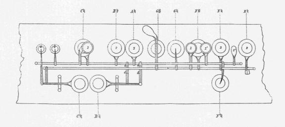
Figure 1: Patent specification drawing for the 1867 Patent flute. The drawing does not include the two extra trill keys often added to the instrument.
