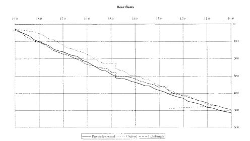
Figure 1: Bore diagrams (X=diameter; Y=length) of three flutes purportedly by John Mitchell Rose.<sup>3</sup> It can be seen that the bores of the two flutes stamped JM Rose (Privately-owned and Edinburgh) are similar whereas the flute stamped J<sup>n</sup>. Rose (Oxford) differs markedly from the others.
