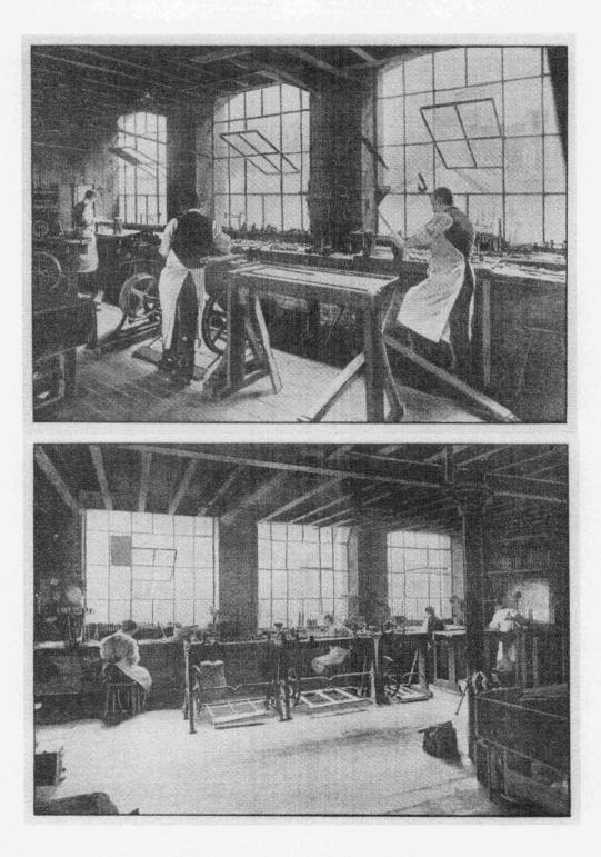
The top picture shows a pole lathe with its poppet heads removed. The L-shaped treadle arrangement on the floor is visible. To the right of the lower picture is an antediluvian lathe with a wooden support, and next to that appears to be the remains of a wooden pole lathe. Pole lathes would have been considered out of date as early as 1850. These workshops show little sign of recent investment.
