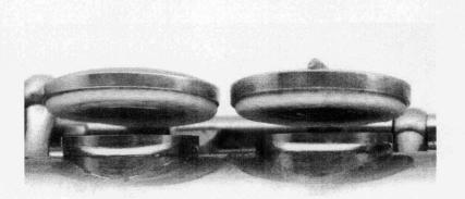
Figure 1: Toneholes on a 'New Metal' (Monel metal) flute, showing the rings soldered onto the toneholes as it was impossible to roll over the edge of the toneholes.
