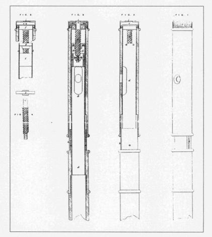
Figure 2: Drawing attached to Rudall & Rose's specification for the Patent headjoint of 1832.
