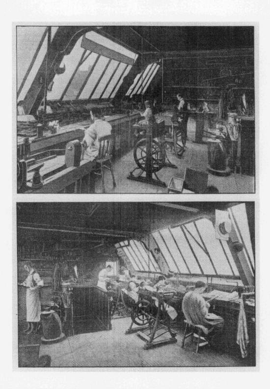
At the left of the top picture is what appears to be a pole lathe made with wooden bearers. The lathe at the far end of the top picture is a triangular-bedded machine dating from the first half of the nineteenth century. These hand lathes are not supplied with slide rests. Each workbench is supplied with a gas burner.
