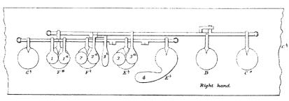
Figure 17: Drawings from the specification for Carte's 1875 Patent flute.
