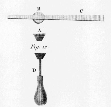
Figure 2: Undercutting tool (fraise), detail from Plate XI of Bergeron's *Manuel du Tourneur*, 1816. The fraise A, threaded in the centre, is inserted into the flute using the tool BC and is picked up on the threaded handle D. Rotating the tool undercuts the hole in a regular and repeatable manner.
