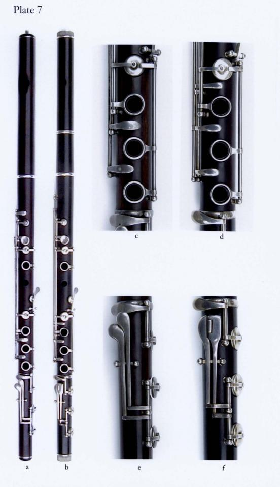
a: 1832 system flute by Boehm. b: 1832 system flute by Rudall & Rose (number 5).c: Boehm right hand mechanism (detail). d: Rudall & Rose right hand mechanism (detail).e: Boehm footjoint (detail). f: Rudall & Rose footjoint (detail).
