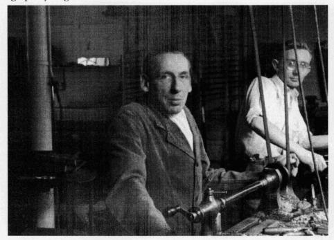
Ted Robbins, the principal woodturner (left) with Charlie Rogers. Ted Robbins is shown using hand tools to turn a cylindrical body joint for a flute. Such an operation would have been more efficiently carried out using a slide rest on an engineering lathe. There appears to have been little investment in the time since the 1913 photographs beyond the provision of a powered overhead shaft to drive the flat belt to the lathe. Photograph by Roger Charters.
