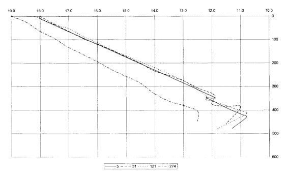
Figure 3: Bores of four Rudall & Rose or Rudall, Rose & Carte 1832 Boehm system flutes. (X=diameter, Y=length) Numbers 5, 31 and 121 have body section bores virtually identical to those of Boehm shown in Figure 4. Number 274, stamped Rudall, Rose & Carte, is a later instrument with Rose's enlarged bore.
