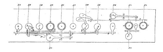
Figure 1: Drawing from Carte's patent specification for the 1851 flute. The note names refer to the note emitted from the hole, not to the finger that is depressed to produce the note.
