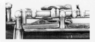
Figure 11: Spencer's horizontal lever operating the D sharp key.
