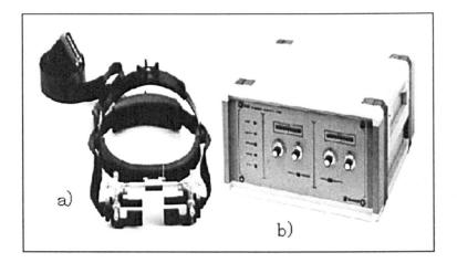
Figure 3.10: IRIS 6500 Eye-tracker and Headset (Skalar Medical BV)
