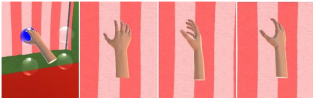
Fig. 2. Demonstration of the virtual hand (set here to size 12cm). From left: hitting a bubble, palm facing down, and palm facing left at approx. 90° and 45° tilted up.
