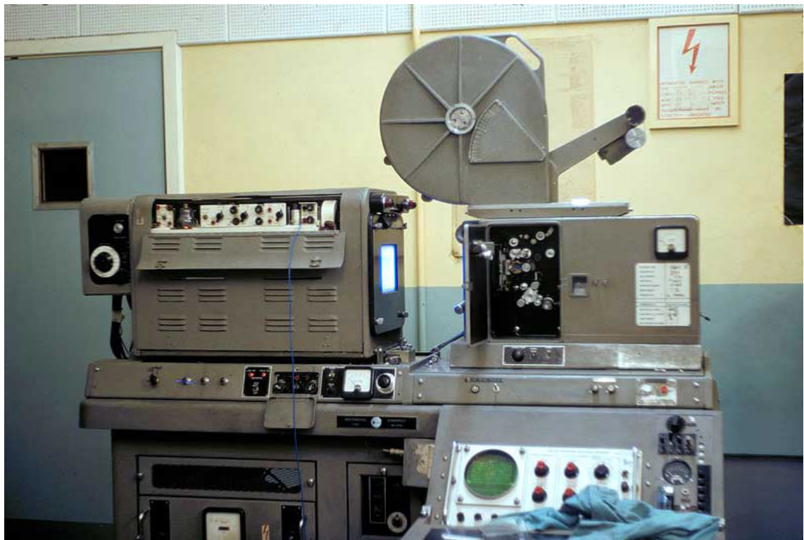
2.2.148 35mm cinema camera used to reconstruct the images received from the Lunar Orbiters on the ground in the Earth Stations
