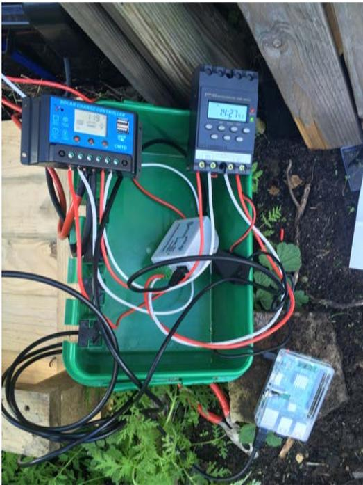
The internal hardware, solar controller, timer, PoE injector, Raspberry Pi 3b.
