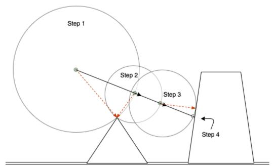
Figure 7.3 Raymarching process [diagram based on Pharr (2005: Fig 8-5)].
