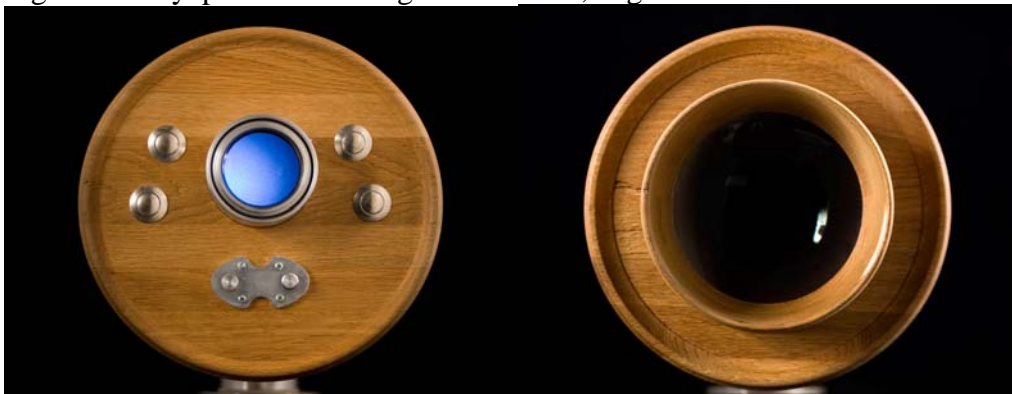
Fig.3. Left: eyepiece with navigation buttons; Right: front lens
