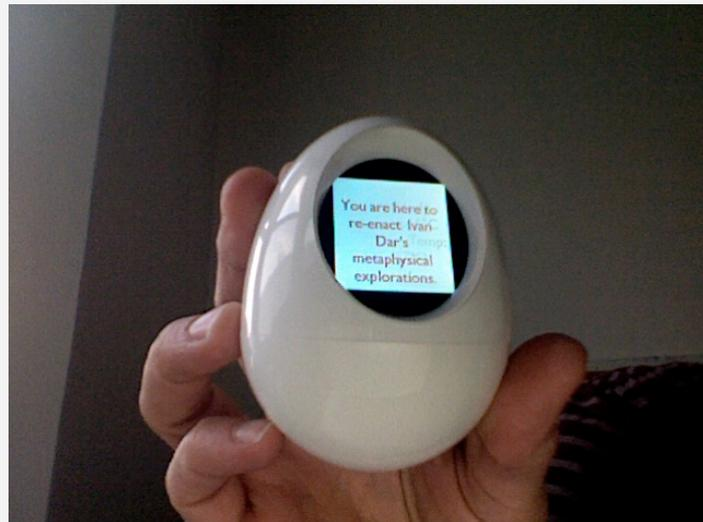
The egg image-display device. It displays content which is generated by the software and then uploaded into it.
