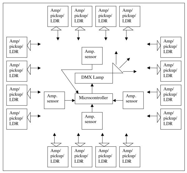
Figure 11. Light Loop structural diagram
