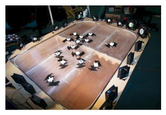
Figure 2: The design of the air-hockey style table containing the monomers. Sails on each monomer are blown by a perimiter of small fans. Another fan below the table passes air through small holes to suspend monomers over the table like small hovercraft.
