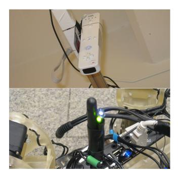
Figure 3: A Nintendo Wii remote provided the location of the robot by tracking the infrared LED mounted on the robot's antenna. The position was measured in pixels and transmitted from the Wii remote to the robot via bluetooth.
