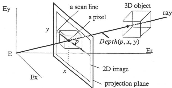
Figure 3.27: Scanline Algorithm Principle.
