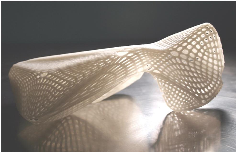
Figure 3.16: Example of a physical model produced with Sintering Rapid prototyping technology, 2007.
