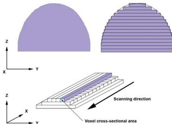
Figure 3.15: Rapid prototyping process
