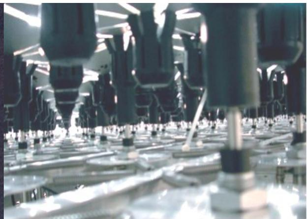
Figure 4.11: *Aegis Hyposurface*, pneumatic actuators.
