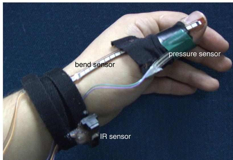
Figure B9: experimental 'glove' with distance, bend and pressure sensors
