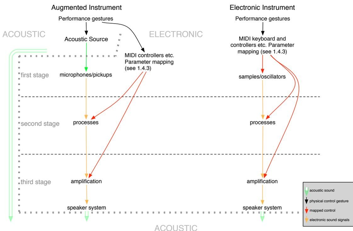
Figure 1.1: Simplified schematic outline of augmented instrument and electronic instrument. This figure is developed further in Chapters 2 and 4 (see figure 2.3 and 4.3).
