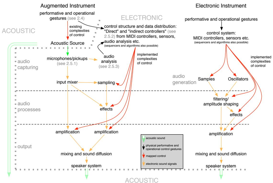
Figure 2.3 Schematic outline of an augmented instrument (based on the simplified Figure 1.1). For comparison a schematic of an electronic instrument has been included to show the difference in the control. The electronic instrument solely relies on the implemented complexities of control while the augmented instrument also ‘inherits’ the existing controls of the acoustic instrument.
