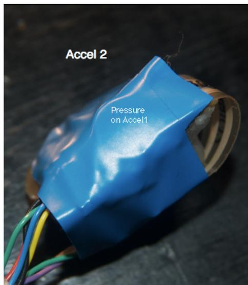
Figure A16: tilt sensor Accel 2 with an additional pressure sensor
