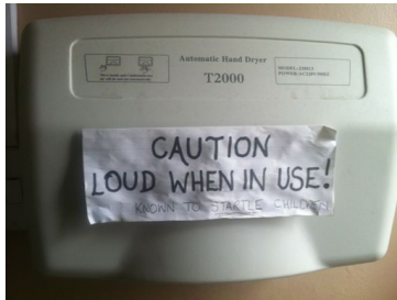
Figure 1: This photo of a Typhoon T2000 is emblematic of this theme. The hand made sign attached to the dryer by the proprietor of a small café, warns: “CAUTION LOUD WHEN IN USE! KNOWN TO STARTLE CHILDREN ”. In contrast to this sign which represents the in situ user’s experience, the product details from the manufacturer state, “low noise 70dB” [9].
